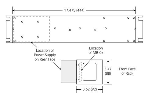
**NOTE** The power supply mounting holes are threaded for 8-32 machine screws. Maximum incursion of screws into mounting holes is 5/16 in. (0.312 in.). It may be necessary to drill additional mounting holes in the RMT-MBBP.
